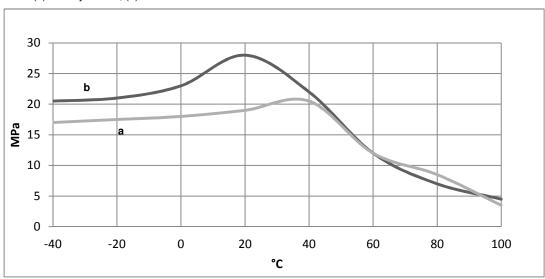
Roller peel test (ISO 4578)(typical average values) - Cure : 16 hours/40°C
