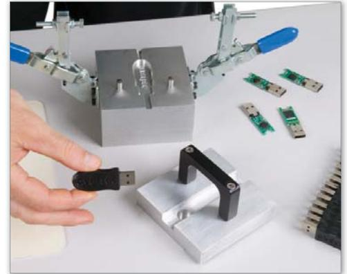
To overmould components using the Overtec system, first open the mould set and place the component inside. Next, load an **Overtec 5 FR** resin stick into an appropriate applicator, like the **Overtec 820-15**, switch on and allow it to reach operating temperature.
