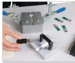
To overmould components using the Overtec system, first open the mould set and place the component inside. Next, load an **Overtec 5 FR** resin stick into an appropriate applicator, like the **Overtec 820-15**, switch on and allow it to reach operating temperature.
