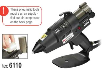
Extremely robust 43mm (1<sup>3</sup>/<sub>4</sub>") pneumatic glue gun with 1000 watt heating for industrial use. Reduces operator fatigue; power-on light; requires air and electric supply. Maximum 7 bar (100psi), for best results set to 4-6 bar (60-90psi) dependent on output requirements.
