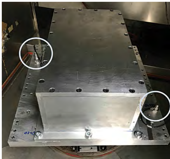
Box shown in vibration testing unit with x, y and z axis sensors
