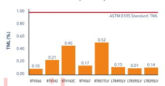
\*Low outgas testing performed using ASTM E595 Low Outgas Test Procedures in a vacuum environment. Test results. Actual results may vary
