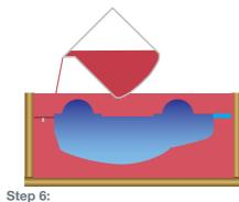
Pour the mixed and degassed silicone to create the 2nd half. It is advisable to vacuum-degas once again after pouring, as some air will enter the silicone while pouring. Allow to fully cure as specified.
