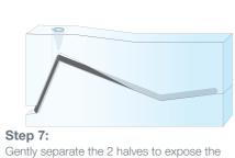
part. Remove the part, the sprue, cast-in air vent
