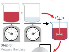
material and catalyst by weight as specified ↑ ↑ ↑ for the grade selected. Mix the components thoroughly, Vacuumdegas the silicone
