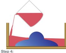
Begin pouring the material, starting first at a low point in the mold. Allow the silicone to cure for the specified time.
