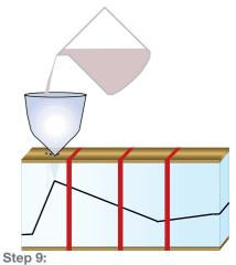
Prepare the casting resin as specified by the manufacturer, pour into the silicone mold via the gate, and allow to cure
