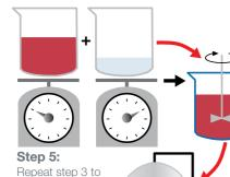
prepare the silicone material for the 2nd ) **† † †** half of the mold.
