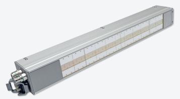
The LED Powerline LC HV is a high-performance UV-LED array for intermediate curing (pinning) and final curing at printing applications. Other application fields are the curing of varnishes or UV reactive adhesives and pottings. Power is supplied via 400 V DC. Separate regulation of each LED segment, e.g. for format size control.
